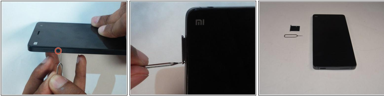
! Check to make sure that the device is powered off.
