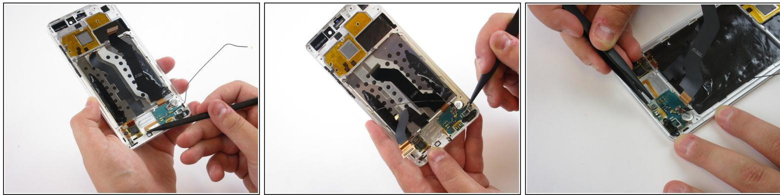
**⚠** The dock connector is firmly adhered to the frame below it. To prevent damage to the phone use minimal force when removing.
