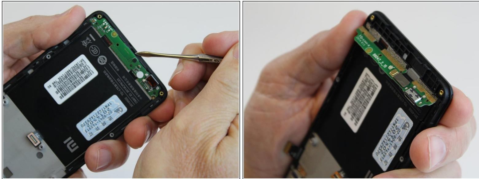
⚠ Do not remove the PCB circuit board at this time.
