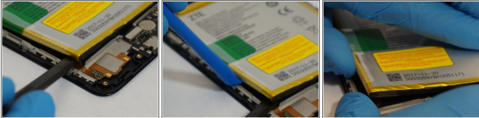
**⚠** Be careful to not damage the battery during this step. If it appears you are using too much force to separate the battery from the frame, you may need to heat the phone to soften the adhesive holding the battery to the phone.
