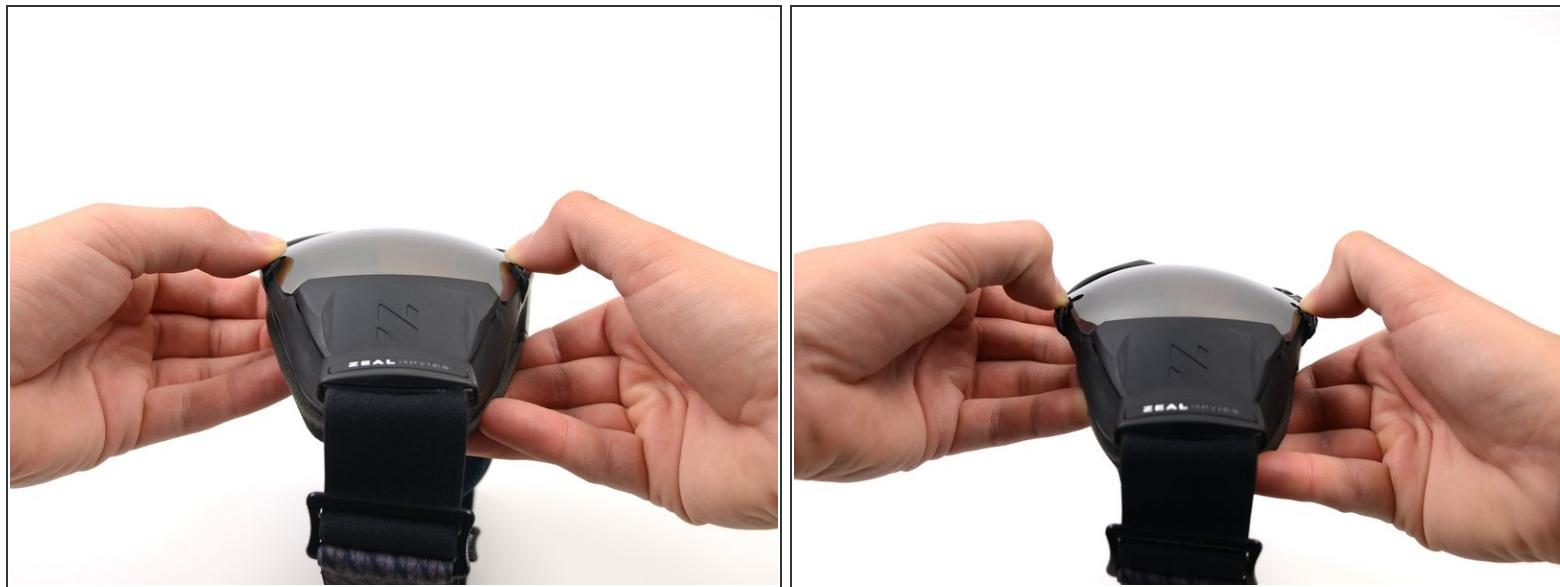
*(i)* In the next few steps, you will be releasing the clips that hold the lens in place. Do not try to completely remove the lens until all the clips have been released.
