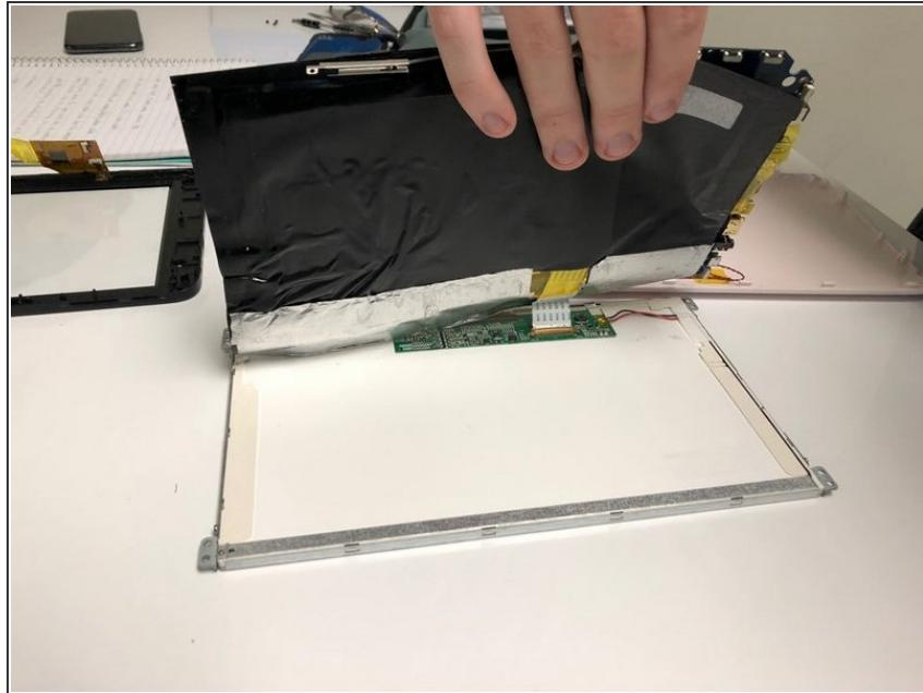
⚠ While you're peeling the adhesive back, be careful because the display is connected by a cable on the right.
