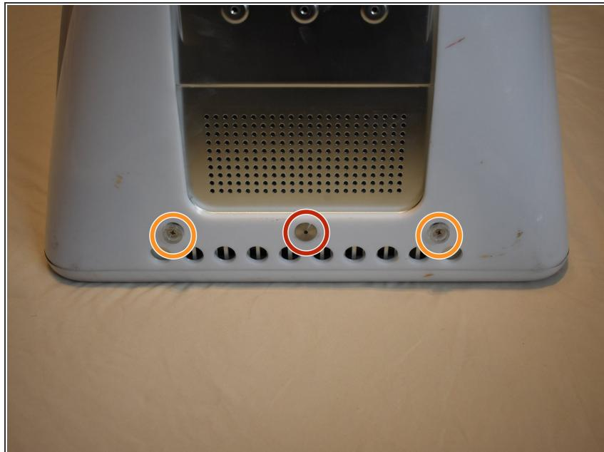
**⚠** Before starting this process it's important to note that the eMac can have some seriously dangerous voltages inside of it, thanks to the CRT display. Before working on an eMac, you should unplug it, press the power button to clear any stored charge on the motherboard, and then let it sit for 24-hours (or more) to allow the CRT to discharge.
