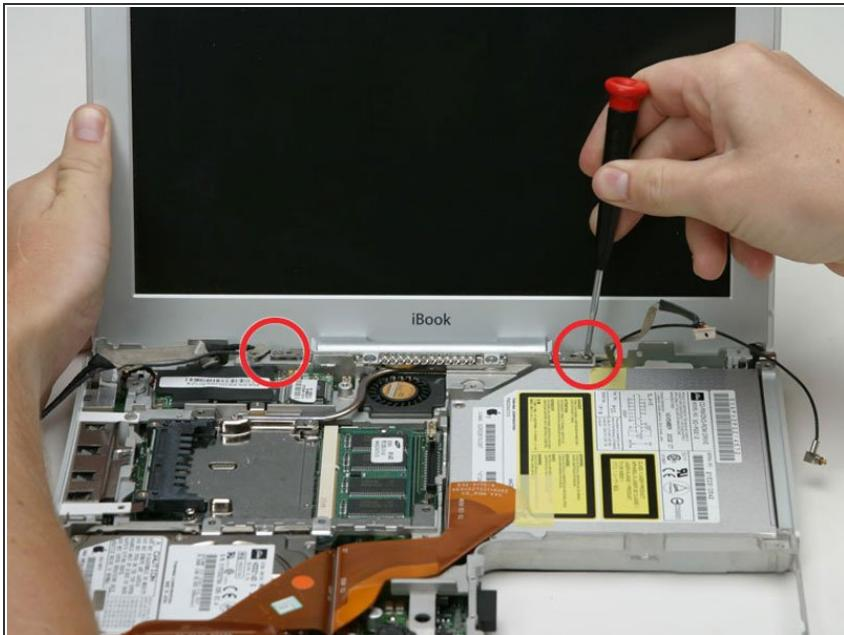
*(i)* Support the display with your free hand while removing the following screws.
