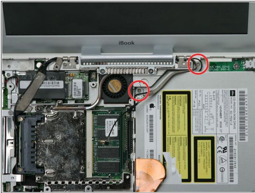
**i** This step may vary on some iBook models. If the screws shown are not on your iBook, you may need to flip the computer over and remove two screws attaching the bottom of the optical drive to the metal framework.
