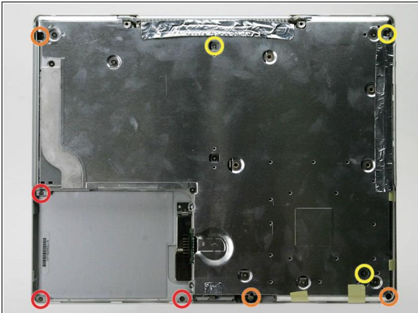
*(i)* All of the screws in the following step have small heads - the screws with larger heads hold the bottom shield on.
