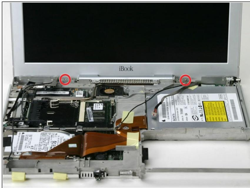
*i* Support the display with your free hand removing the following screws.
