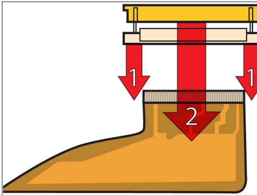
*(i)* This is a diagram of the ribbon clamp connectors you will disconnect in the next step.
