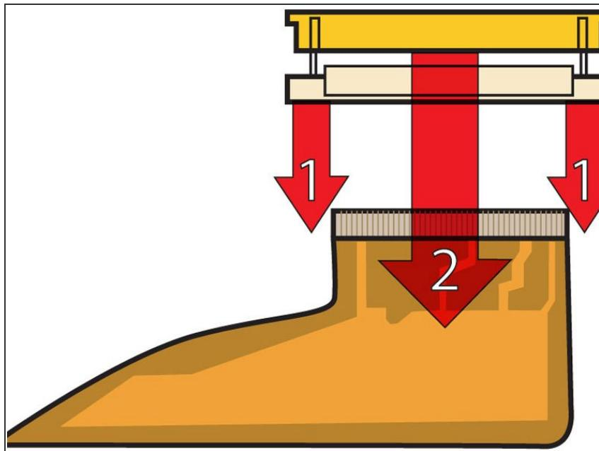
*(i)* This is a diagram of the trackpad ribbon clamp connector you will disconnect in the next step.
