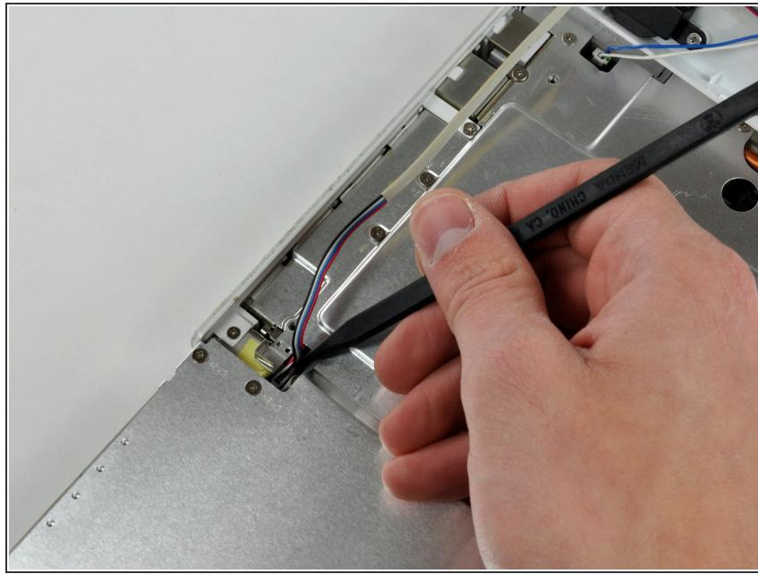
**i** The connectors at the ends of the following cables are attached very firmly to the sockets on the logic board. Pulling directly on the cable will either separate the cable from its connector or the socket from the logic board.
