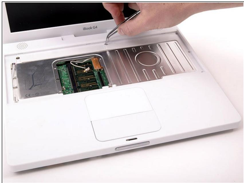
**i** We recommend placing the computer on a slab of grey anti-static packing foam from this point on to prevent damaging the logic board.
