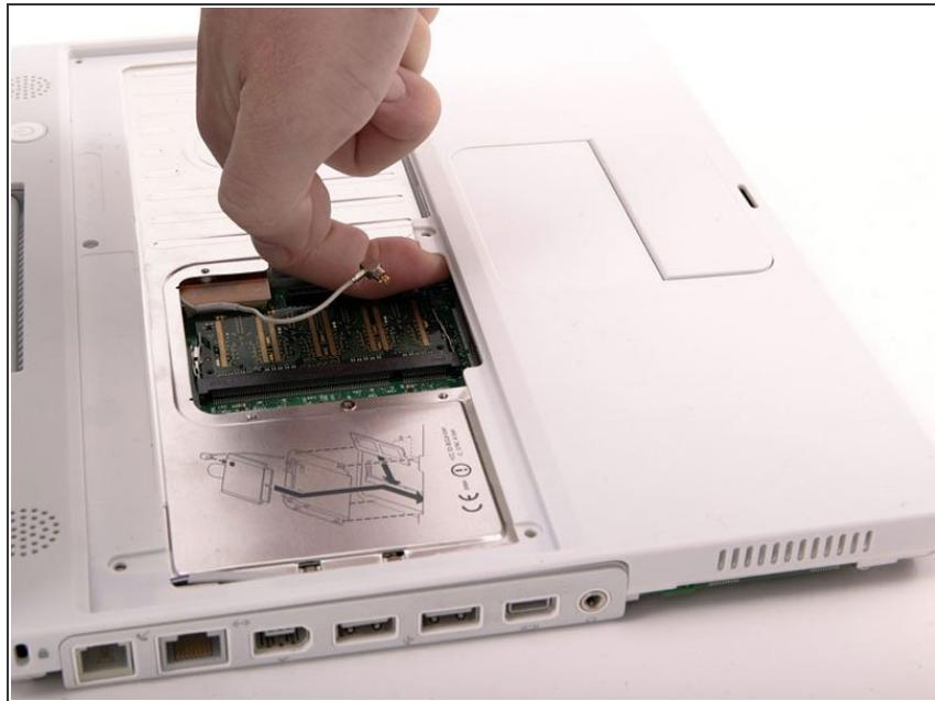
**i** Before you can yank the upper case off, you must disconnect the trackpad connector, the blue and white power cable, and speaker cable as described in the next steps.
