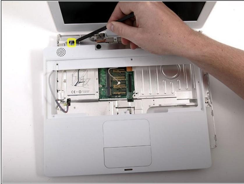
**⚠** The connectors at the ends of the cables are attached very firmly to the sockets on the logic board. Pulling directly on the cable will either separate the cable from its connector or the socket from the logic board.
