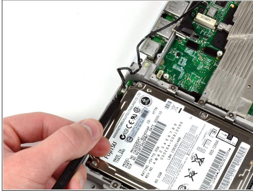
**i** The cable you're about to remove is very fragile - do not pull directly on the wires. Instead, try to pry up the connector directly, using a spudger or a small flathead screwdriver if necessary.
