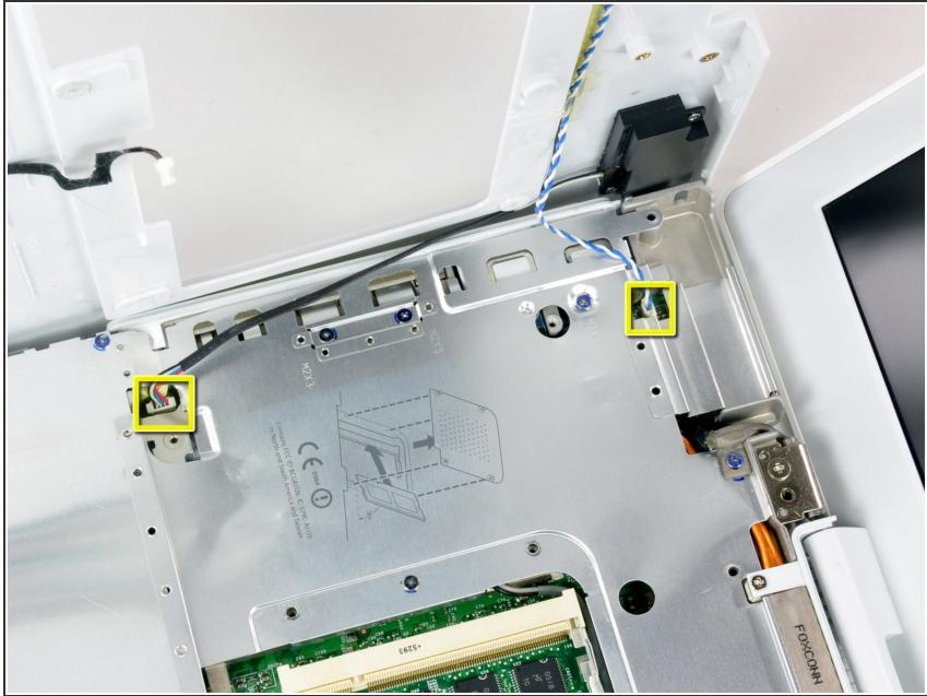
**!** The sockets attached to the motherboards of most iBooks are very weak and easily broken. Use extreme caution when pulling connectors out of their sockets.
