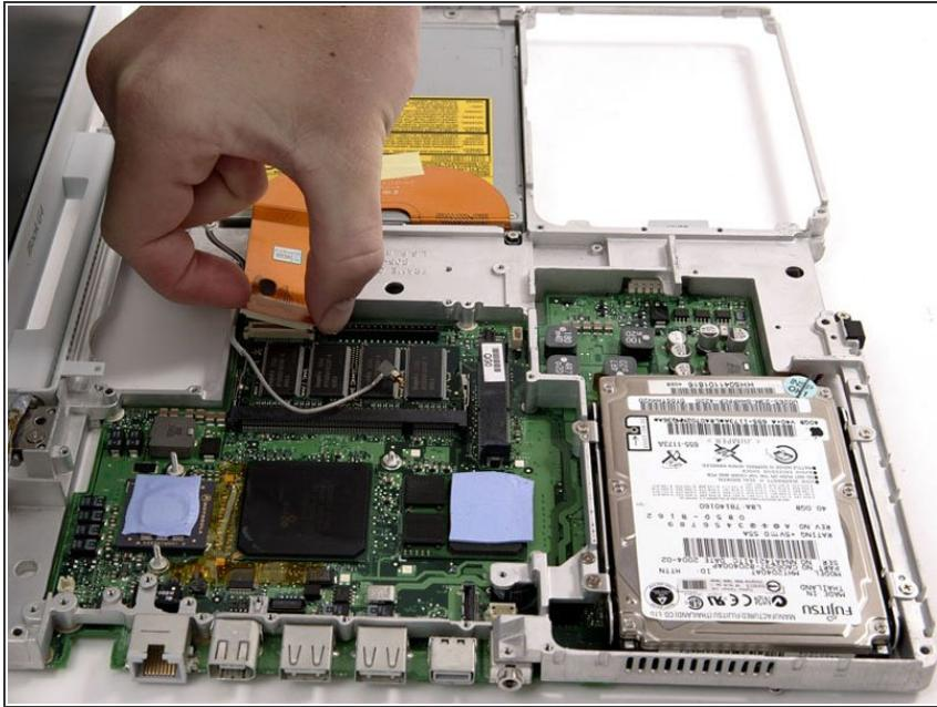
**ⓘ** There are two different styles of optical drive ribbon. If the cable extending from the optical drive is white, skip this step. If the cable is orange, then complete this step and skip the next two steps.
