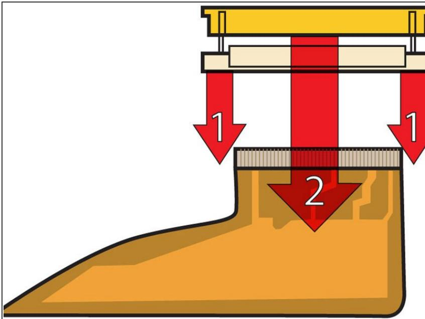
**ⓘ** This is a diagram of the ribbon clamp connector you will disconnect in the next step.
