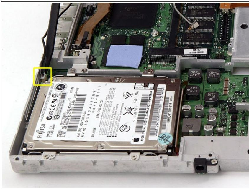
⚠ The cable you're about to remove is very fragile - do not pull directly on the wires. Instead, try to pry up the connector directly, using a spudger or a small flathead screwdriver if necessary.
