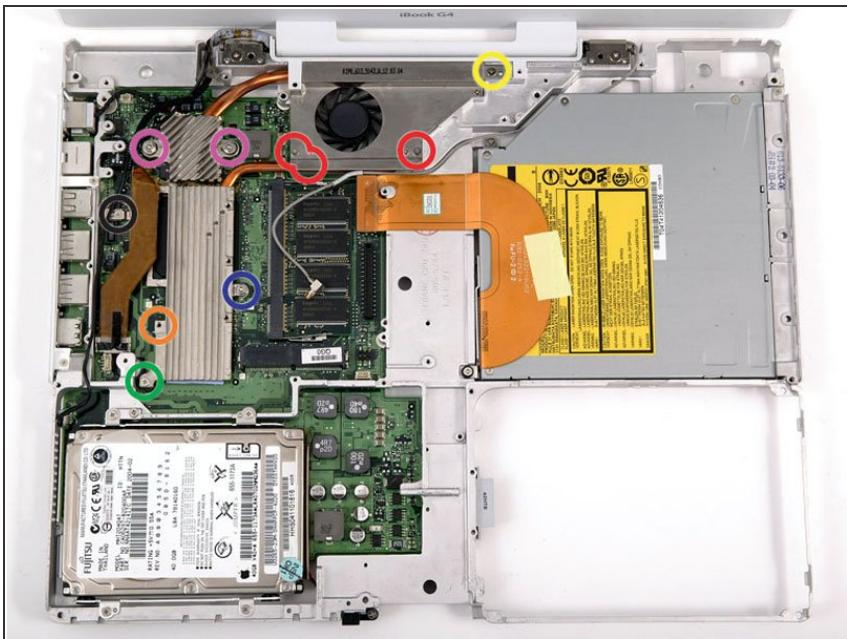
Due to variations between iBook G4 models, your heatsink may have either 5 or 6 screws. We've noted all possible positions for screws in the step below. If there's no screw to remove, then skip to the next screw. Be sure that you remove all necessary screws before attempting to remove the heat sink.
