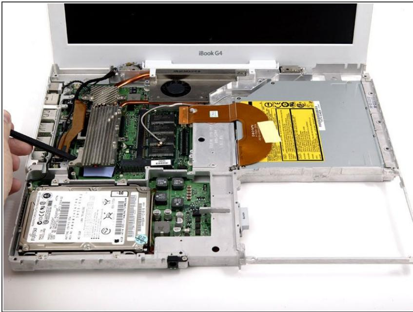
**i** It may be necessary to soften the thermal paste between the logic board and heat sink. You can soften the thermal compound using a hairdryer. Move the hairdryer back and forth over the ribbed metal section of the heat sink for one minute. At this point, the heat sink should come free easily.
