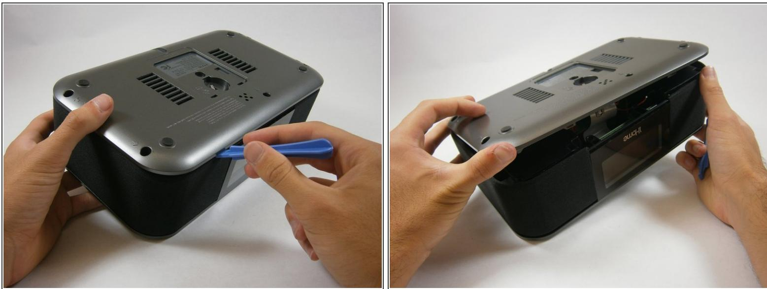
**⚠** The bottom cover is attached to the back cover by two plastic clips. Don't use excessive force.
