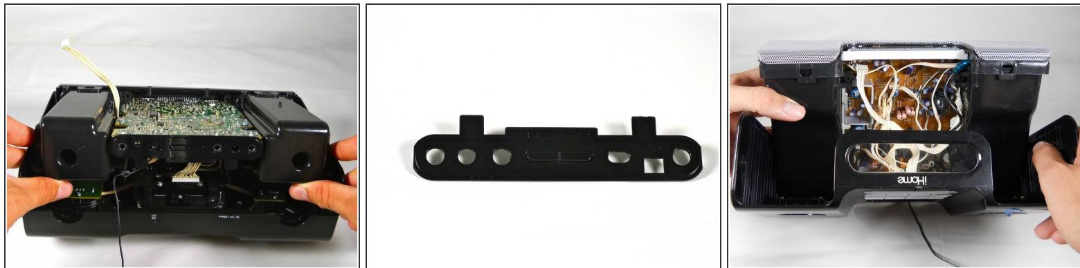
! Carefully pull up on speaker boxes to pry them loose from the bottom case. Wires attach the underside of the motherboard to the upper case, and they will not separate completely at this time.
