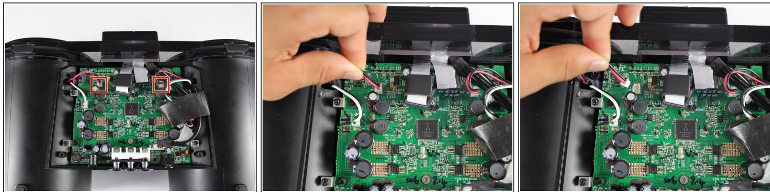
**(i) Both speakers should be removed at this point.** If only one speaker has been removed, follow steps 12-14 of this guide to remove the other speaker.
