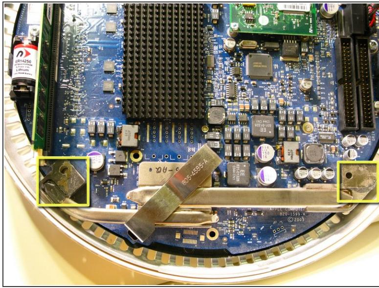
**⚠** Important information for reassembling your iMac. You must clean and apply thermal paste to the mating surfaces of the CPU Heat Pipe and The Upper Housing, indicated by the yellow squares in the 2 photographs. Follow iFixit's excellent Thermal Paste Guide [How to Apply Thermal Paste](#).
