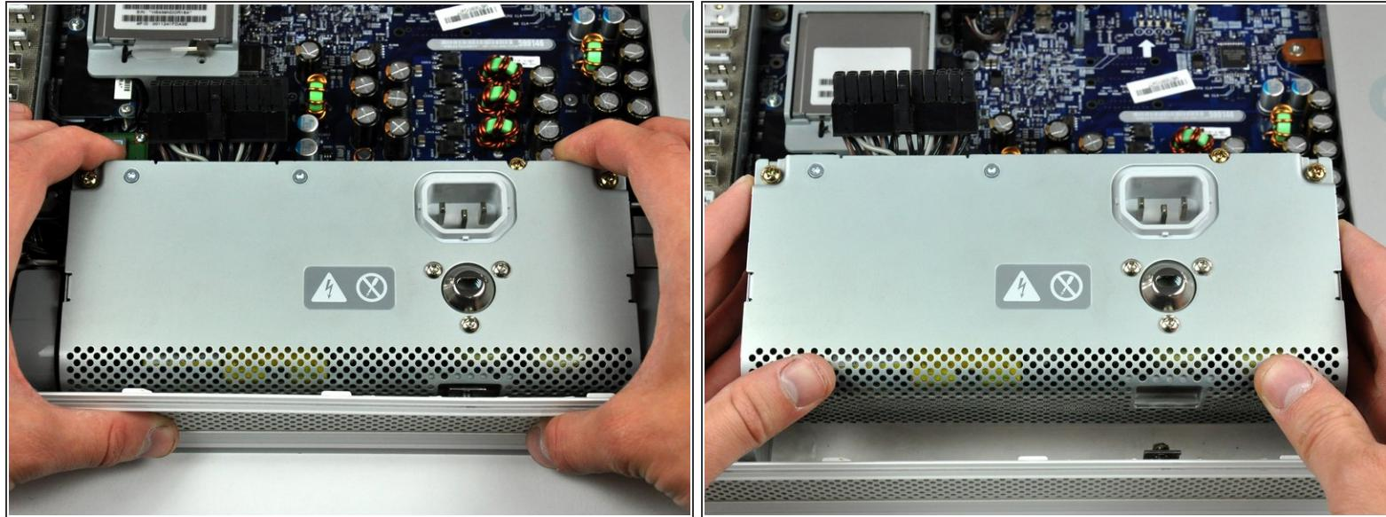
**⚠** There are several capacitors mounted to the logic board in close proximity to the power supply. Try not to disturb them, as they are delicate and may break off the board.
