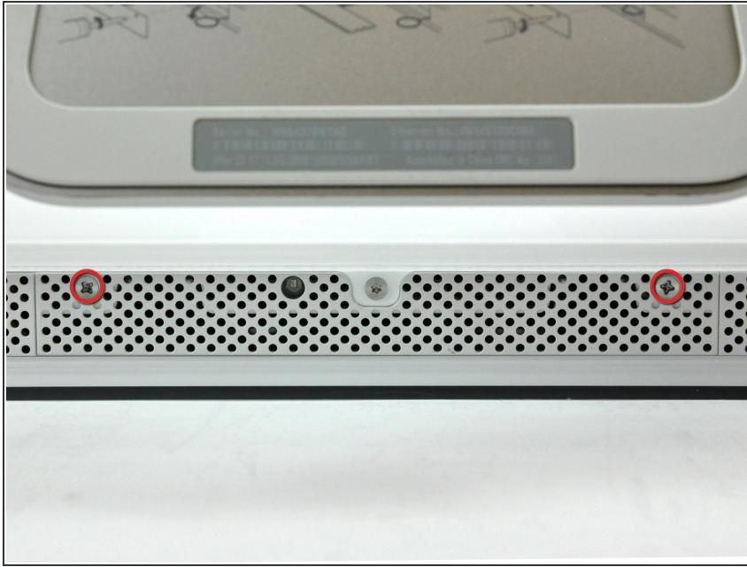
**⚠** Before you work on the computer, unplug the computer and press the power button for 20-30 seconds to drain the stored energy in the power supply.
