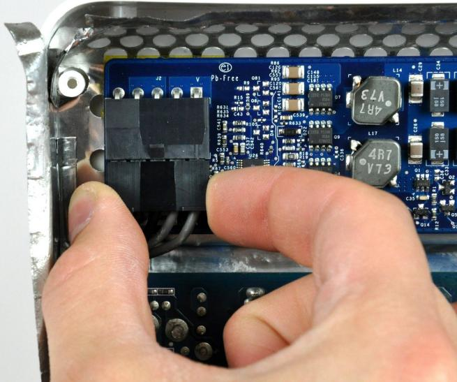
**⚠** The next few steps bring your hands close to the exposed face of the power supply. **Do not** touch the face of the power supply to avoid a high voltage shock from the many large capacitors attached to the board.
