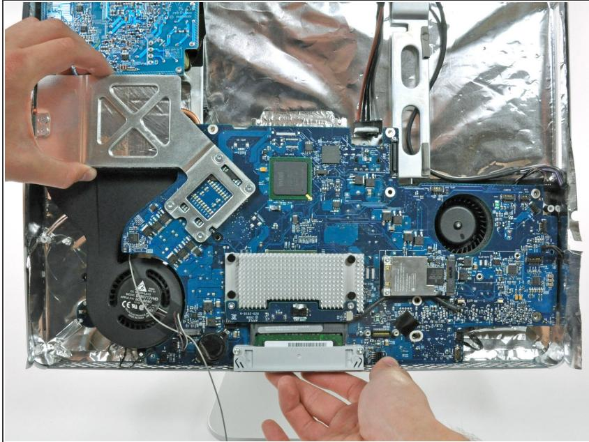
**⚠** Be sure to touch the chassis before proceeding to discharge any static.
