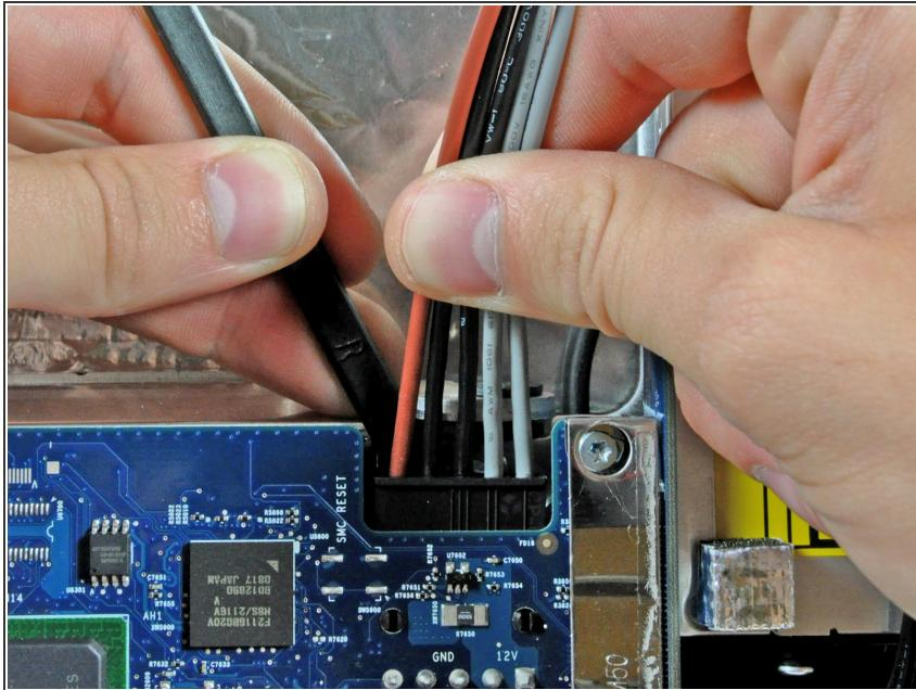
**⚠** The next few steps bring your hands close to the exposed face of the power supply. **Do not** touch the face of the power supply to avoid a high voltage shock from the many large capacitors attached to the board.
