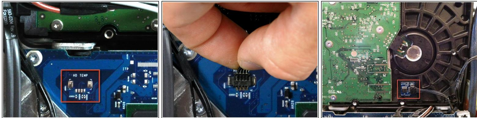
**⚠** A hard drive thermal sensor may be present on some models. If your logic board is missing the hard drive thermal sensor socket highlighted in red in the first picture, skip this step.
