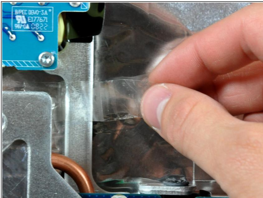
**i** If necessary, remove the piece of tape holding the AC-in cable under the chassis.
