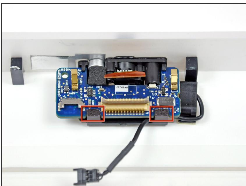
*(i)* Rather than being held down by screws, the camera board is held down by a black plastic bracket attached to the front bezel.
