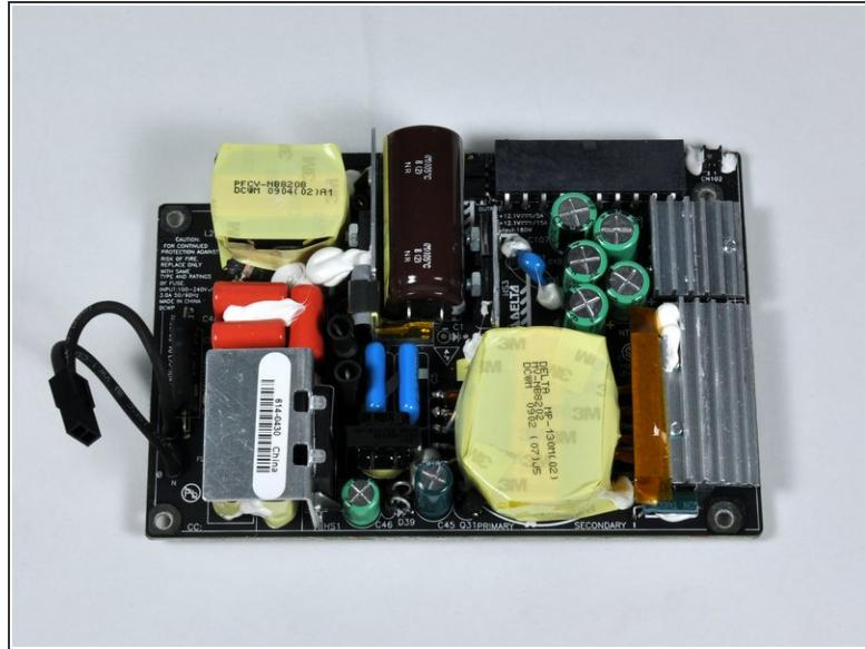
**⚠ This is the power supply. If you're doing this at home, **be very careful handling it, as capacitors can remain charged even after power has been disconnected from the computer.****
