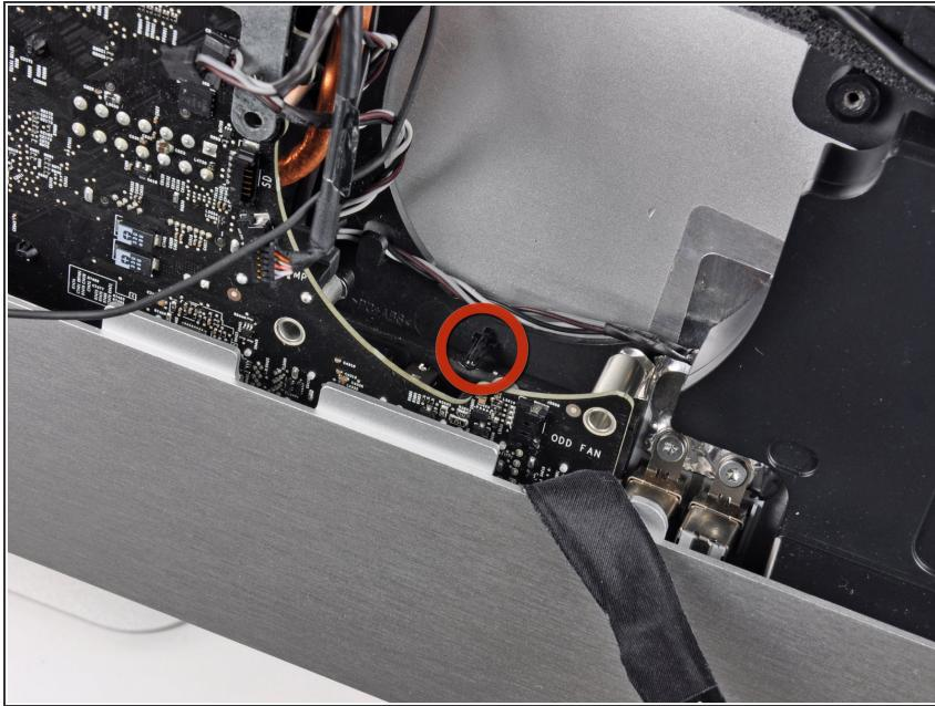
**⚠** In the following steps, you will maneuver the logic board out from the outer case. In doing so, be aware of the many cables still attaching the logic board to the outer case.
