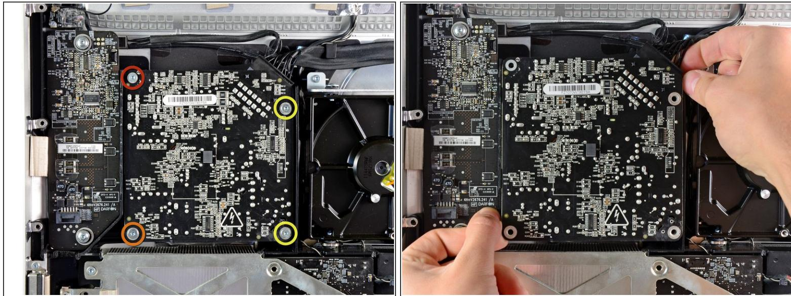
**⚠** Be careful not to touch any solder joints on the back of the power supply. Capacitors may be charged enough to give you a dangerous shock.
