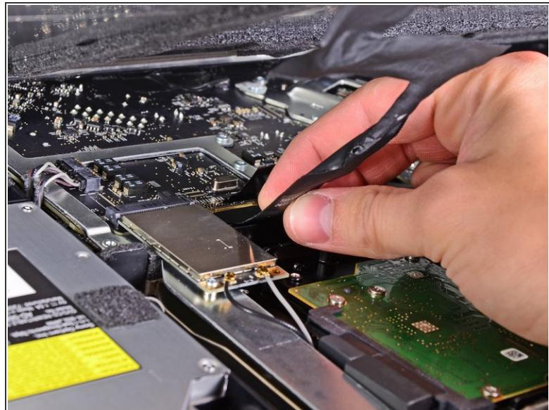
**⚠** The display data cable plug has a wire lock. Disengage the plug's lock by rotating the plastic tab so that it points upward. (It is not a pull tab.)
