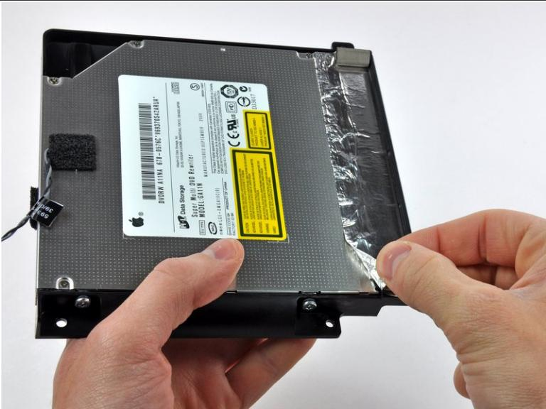
**i** It is not necessary to peel all of the EMI tape off the optical drive bracket. Only peel up the portion highlighted in red that is attached to the body of the optical drive.
