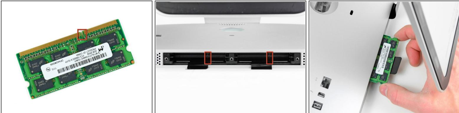
**⚠** When installing new RAM modules, it is important to orient them correctly.
