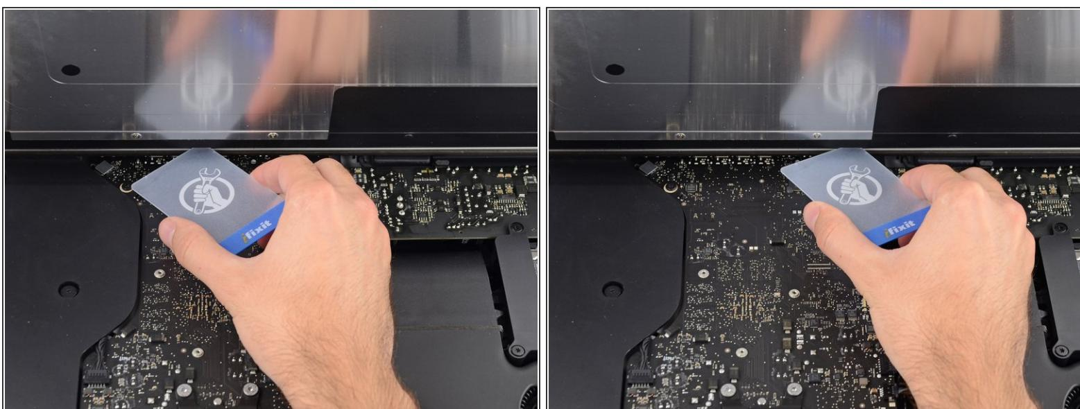
*(i)* If necessary, a plastic card can be used to cut any remaining sections of the bottom adhesive strip.
