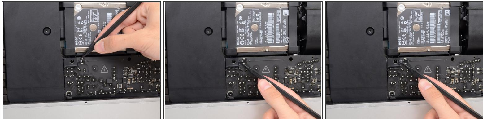
⚠ The next few steps bring your hands close to the exposed face of the power supply. **Do not** touch the face of the power supply to avoid a high voltage shock from the many large capacitors attached to the board.
