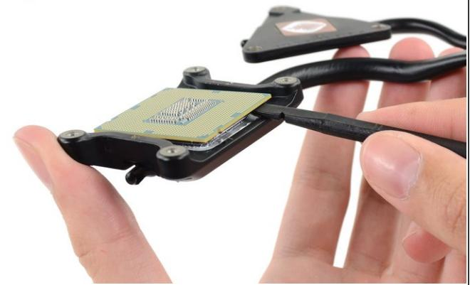
*(i)* The CPU will most likely be stuck to the heat sink with thermal compound.
