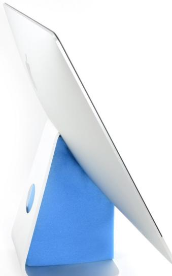
**i** With the hinge free to move, the iMac will be unbalanced and hard to work on. Repairs can be completed as shown, but are faster and easier with an [iMac service wedge](#).
