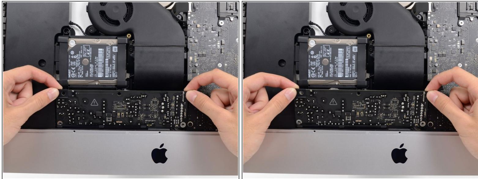
**⚠** When working on the power supply, **be very careful** not to touch the capacitor leads or any exposed solder joints on the back of the power supply. Only handle the board by the edges.
