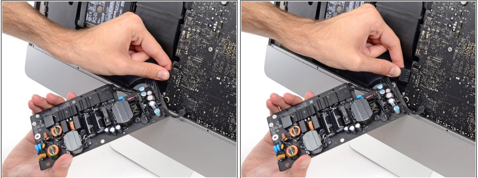
**⚠️ Be very careful** not to touch the capacitor leads or any exposed solder joints on the back of the power supply. Only handle the board by the edges.
