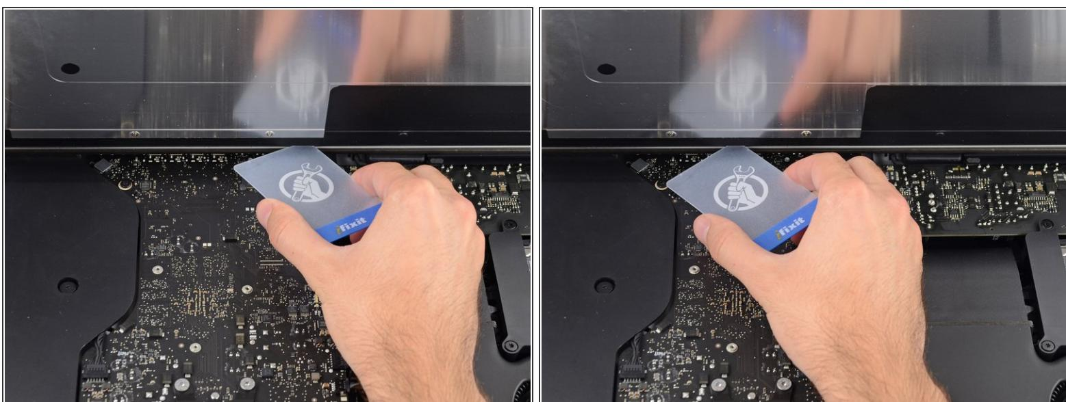
● If necessary, a plastic card can be used to cut any remaining sections of the bottom adhesive strip.
