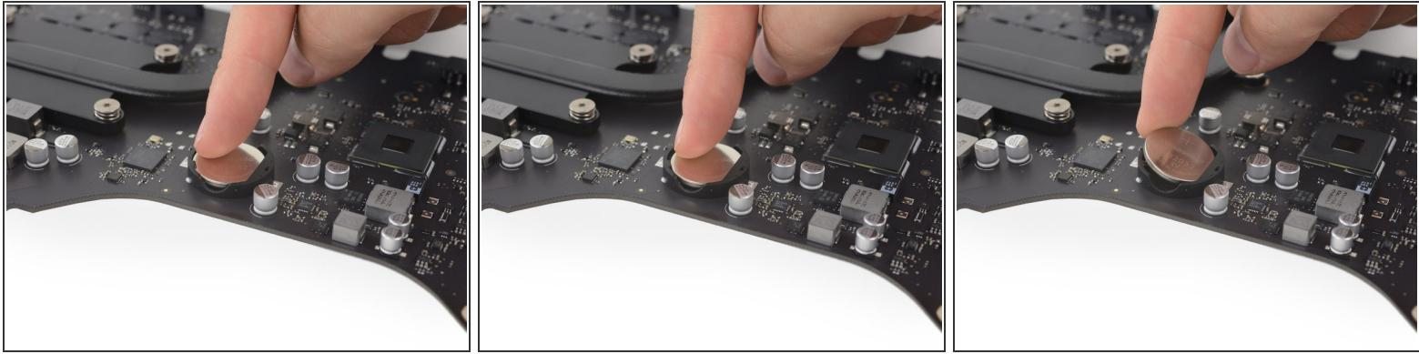
*(i)* The PRAM battery is secured by a spring contact and two small plastic nubs.
