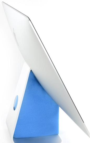
**i** With the hinge free to move, the iMac will be unbalanced and hard to work on. Repairs are fast and easy with an [iMac service wedge](#), but can be completed without one.
