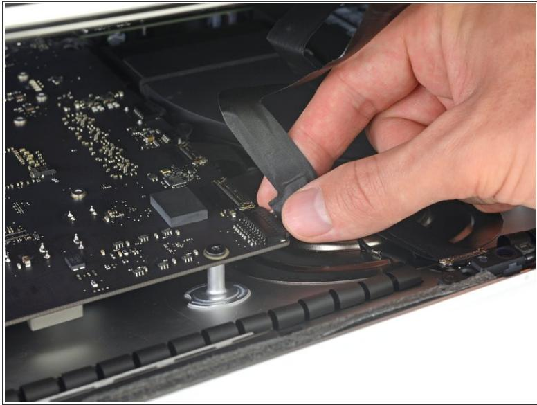
*(i) At this point it's a good idea to test your repair, in order to make sure your iMac works properly before you seal it back up. Follow the next three steps to temporarily reconnect the display cables and boot up your iMac prior to pulling the protective film off the adhesive strips.*
