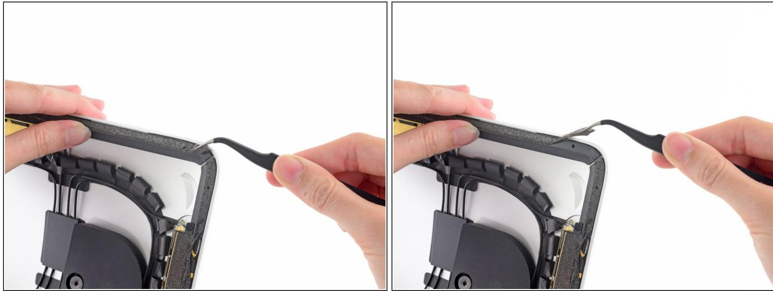
**⚠** Before you start placing strips, remove all of the old adhesive around the perimeter of the rear enclosure.
