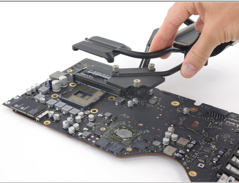
! Note that the CPU will most likely remain stuck to the underside of the heat sink as it's lifted out. Take care not to damage it.
