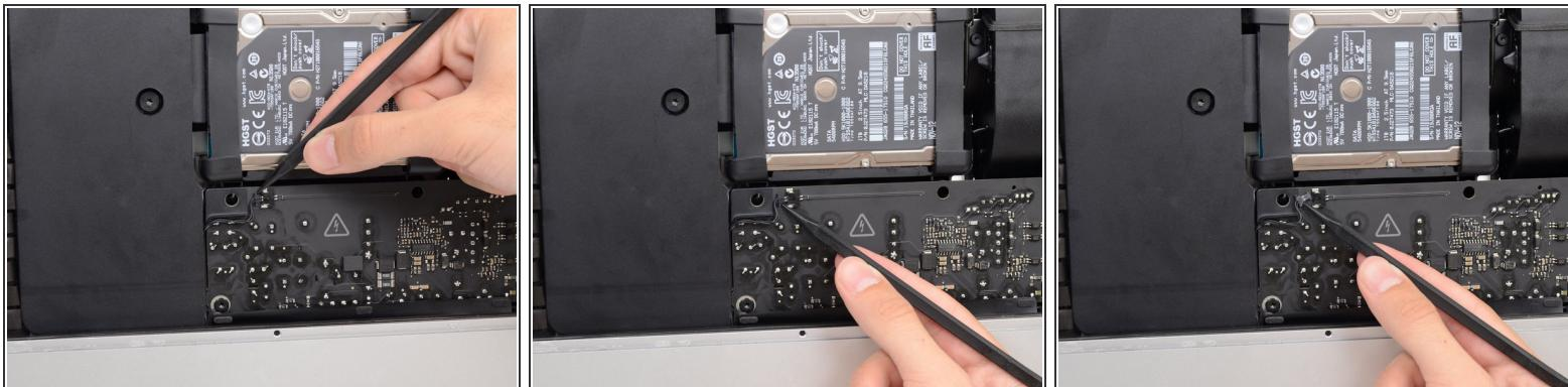
! The next few steps bring your hands close to the exposed face of the power supply. **Do not** touch the face of the power supply or any of the exposed solder. Touching it risks a high voltage shock from the many large capacitors attached to the board.
