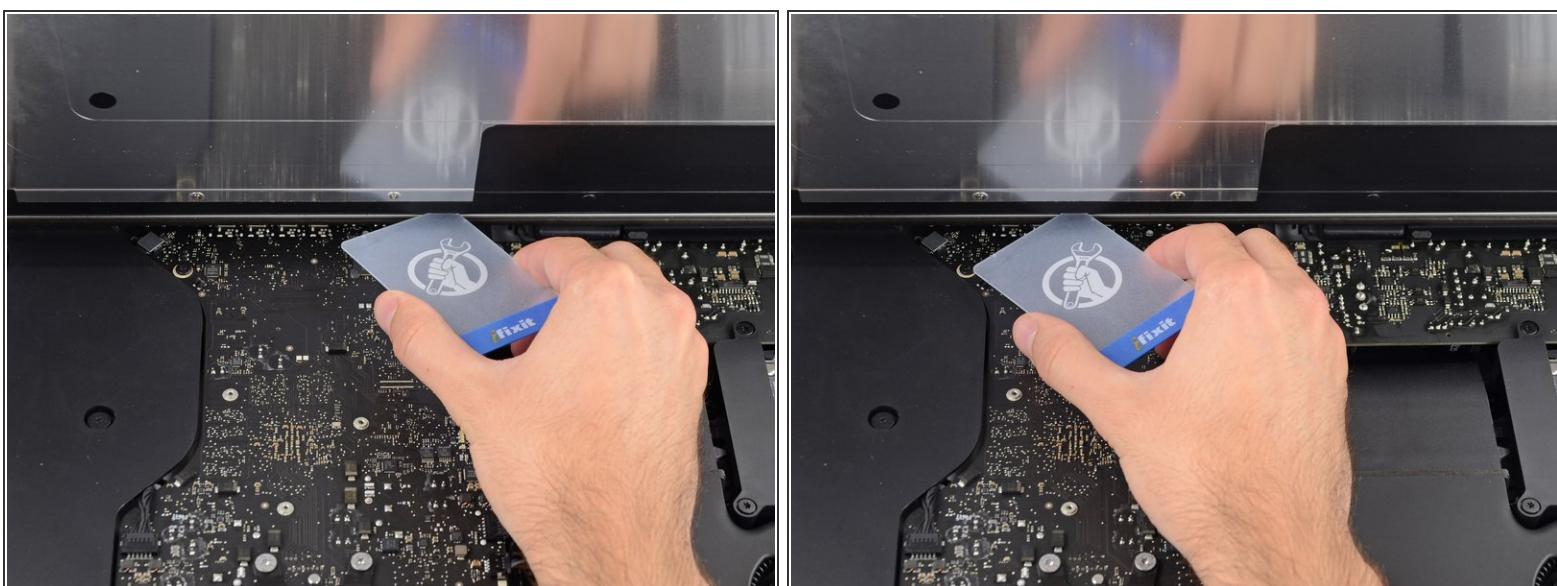
● If necessary, a plastic card can be used to cut any remaining sections of the bottom adhesive strip.
