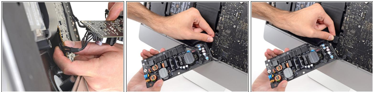
**⚠** **Be very careful** not to touch the capacitor leads or any exposed solder joints on the back of the power supply. Only handle the board by the edges.
