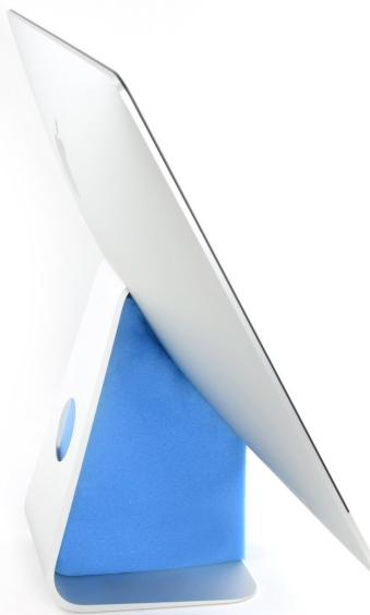
**i** With the hinge free to move, the iMac will be unbalanced and hard to work on. Repairs are fast and easy with an [iMac service wedge](#), but can be completed without one.
