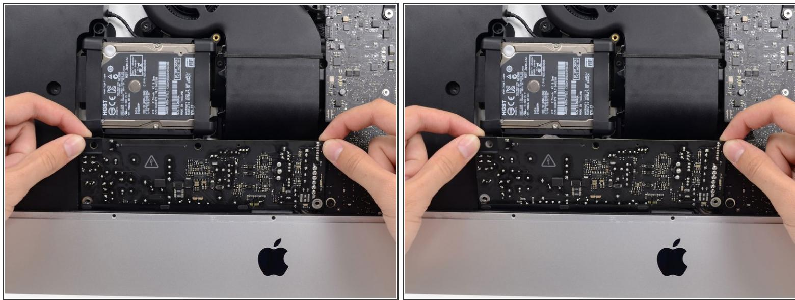
**⚠** When working on the power supply, **be very careful** not to touch the capacitor leads or any exposed solder joints on the back of the power supply. Only handle the board by the edges.
