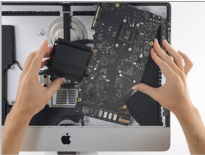
**⚠** When removing and installing the logic board, take care not to damage the delicate [microphone ribbon cable](#) at the bottom left.
