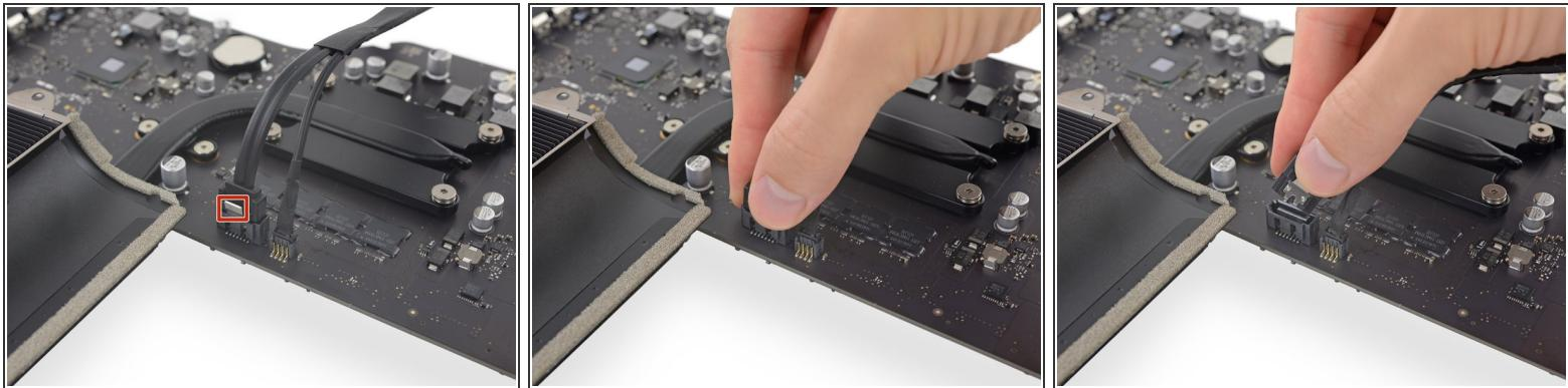
ⓘ The SATA data connector has a clip that must be pressed to allow removal.
