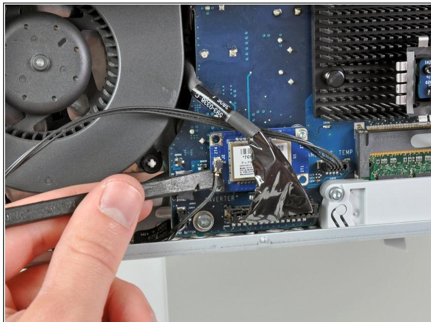
**i** The Bluetooth Board is located on the lower left corner of the iMac, to the left of the RAM modules.
