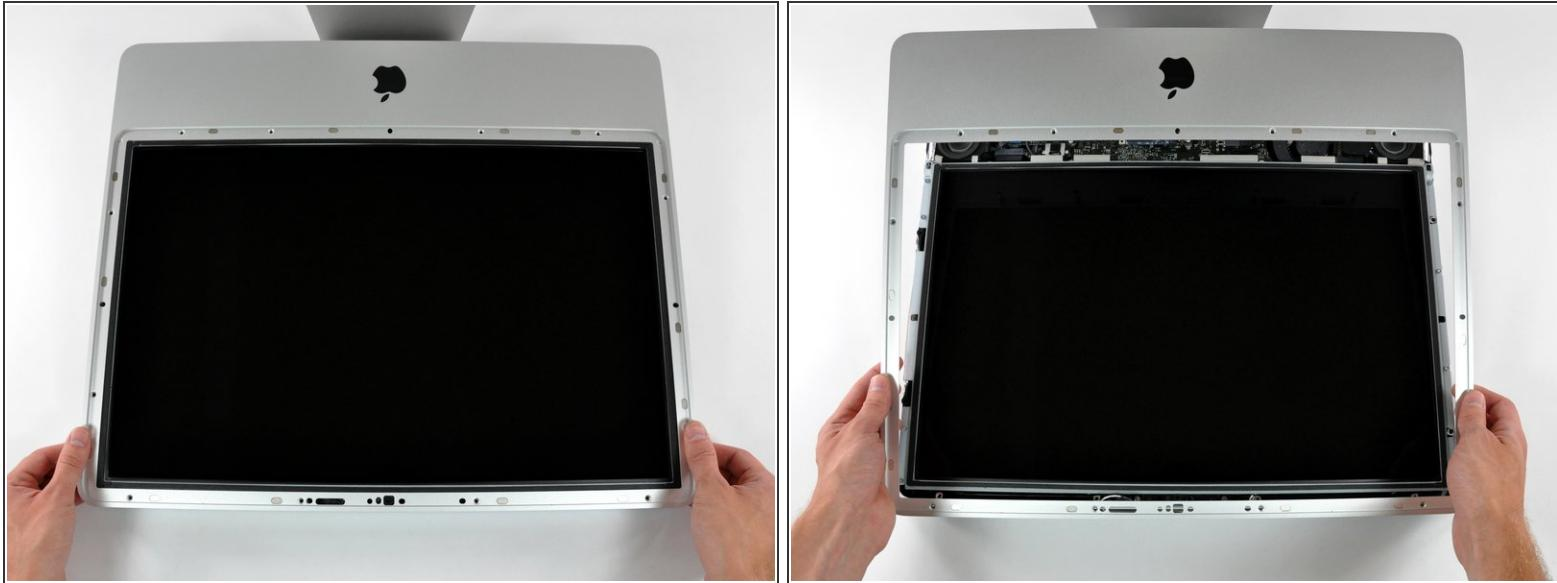
⚠ The front bezel is still attached to the iMac by the microphone cable.
