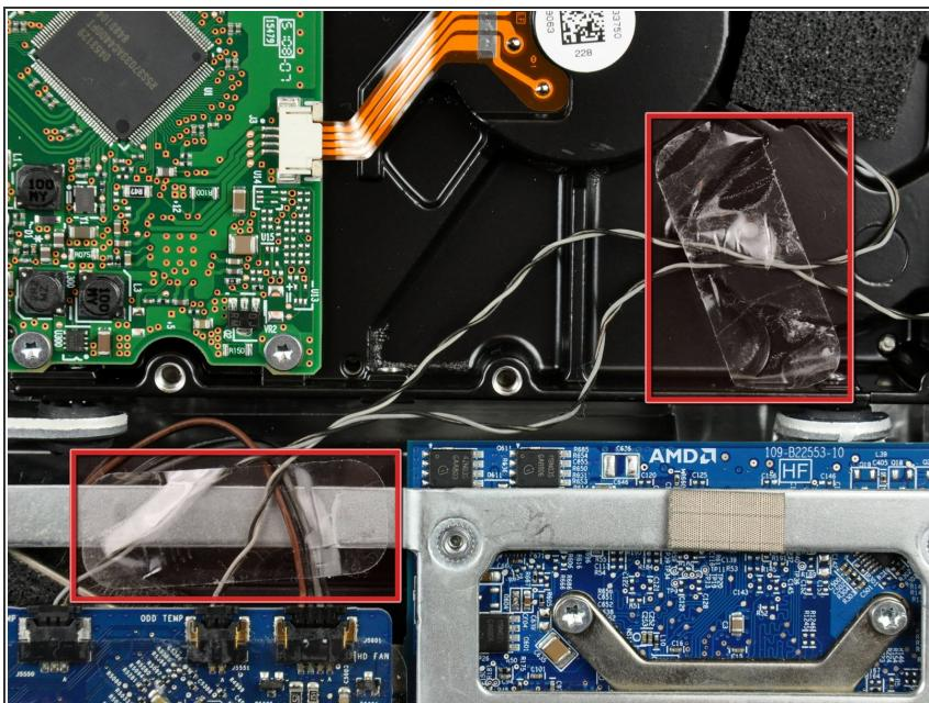
*i* If necessary, remove the pieces of tape securing the hard drive/optical drive thermal sensor cables to your iMac.
